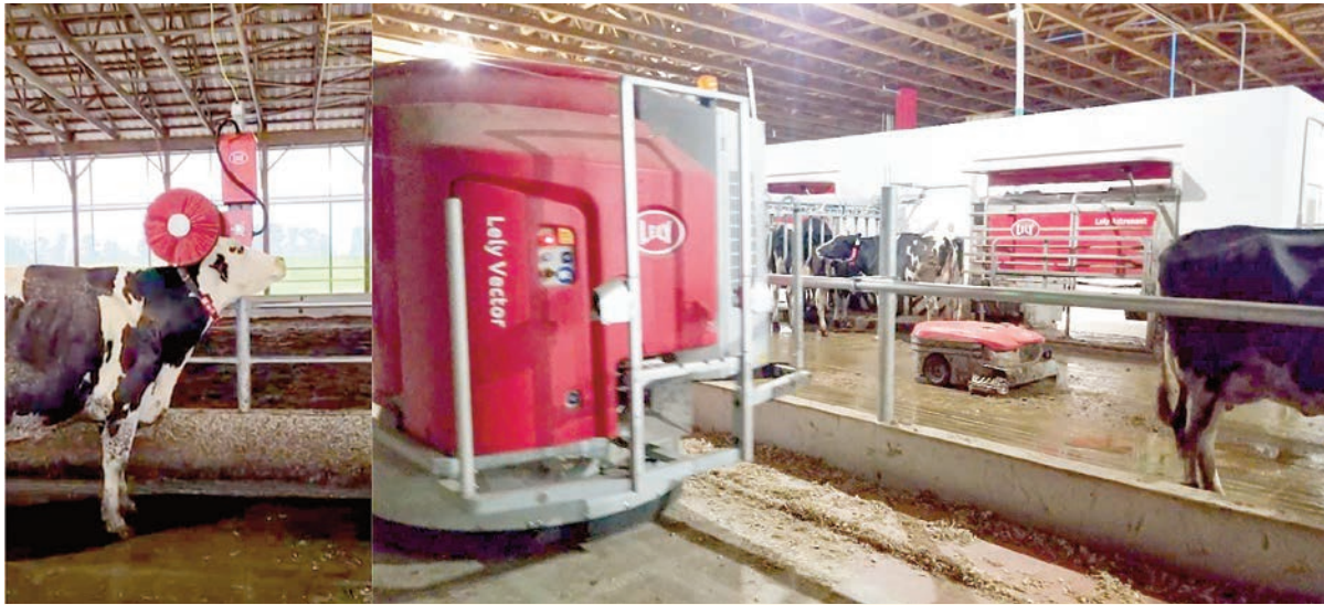
Robotic systems for milking and feeding -- as well as grooming -- are shown here at Oakleigh Farm, Mercersburg, Pennsylvania. The dairy features many automated technolo-
