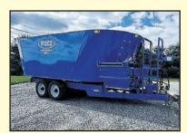
**Patz 950 Twin Screw Mixer** Tub Magnet, Two-Speed, Scale
