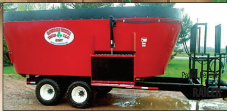
NOW AVAILABLE! CLOVERDALE MODEL 650T T MIXER 825 Total Cu. Ft. Capacity, Twin Auger, 16"-21" Knives for Faster Processing Hay, 2 Speed Gear Box.
